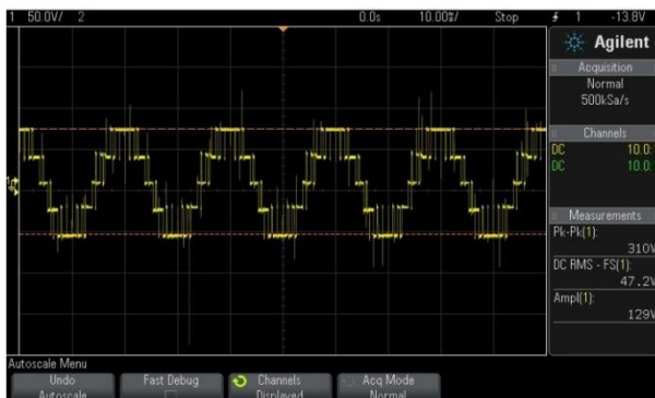
Fig. 18: Output Waveform of Modified Inverter-Fed Drive
