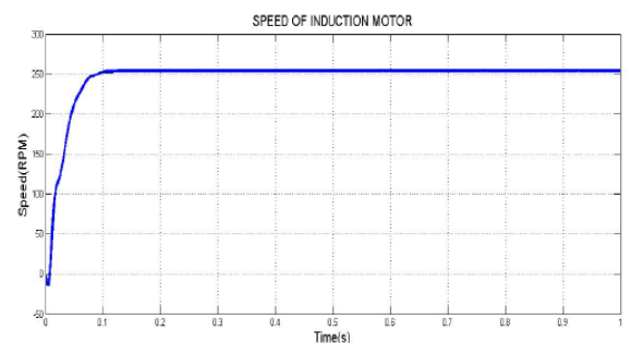
Fig. 8: Speed Response of Conventional Inverter-Fed Drive
